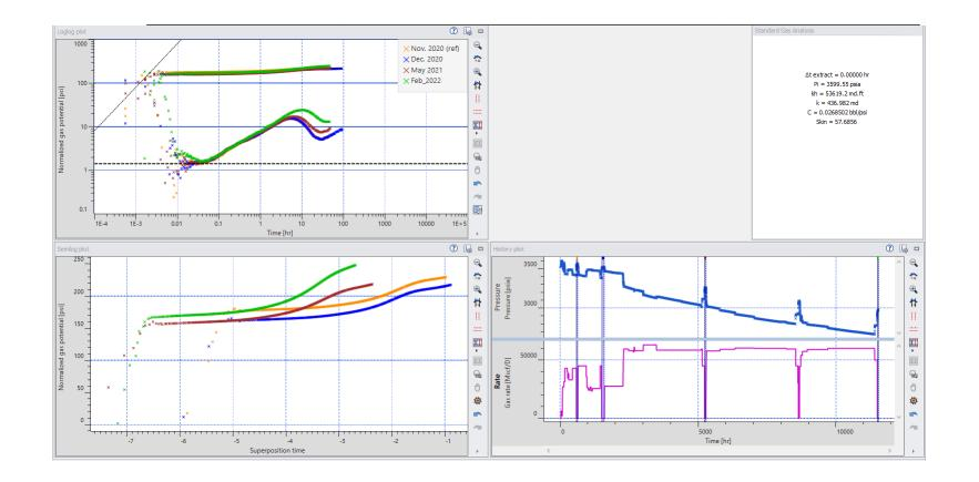
Nov 2020: 1<sup>st</sup> PBU @ 0.8 bcf cum & 35 psi depletion from initial pressure Dec 2020: 2<sup>nd</sup> PBU @ 2 bcf cum & 73 psi depletion from initial pressure May 2021 3<sup>rd</sup> PBU @ 10 bcf cum & 307 psi depletion from initial pressure Feb 2022 4<sup>th</sup> PBU @ 25 bcf cum & 559 psi depletion from initial pressure
