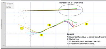
To fine the range of static GIIP a detailed surveillance program was established to acquire pressure points and PBUs to calculate the dynamic GIIP with different techniques including (static material balance, deconvolution, RTA)
